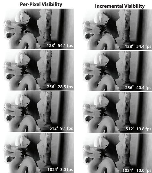
Figure 4: Compare (left) brute force visibility and (right) our incremental refinement. Brute force computations ray march from each pixel to every VPL, whereas incremental computations reuse results from coarser visibility passes.
